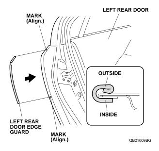
14. Starting at the feature line, use a rubber mallet to tap the left rear door edge guard into position with a series of light taps, then work up and down. Make sure the position of the left rear door edge guard is correct. Once in place, do not attempt to remove, reposition, or reinstall the left rear door edge guard.
